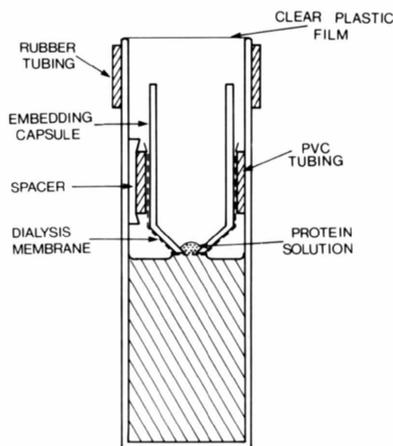
Fig. 1. Sectional drawing of the microcrystallization assembly.
