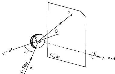
Fig. 1. Experimental arrangement for obtaining a rotation photograph.
