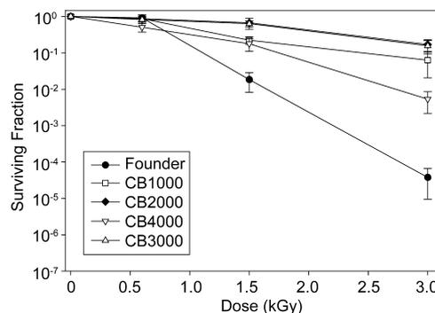
FIG. 2. Survival curves for evolved *E. coli* strains. Survival curves were generated as described in Materials and Methods (also see the supplemental material) for the founder strain and the evolved strains. Results were obtained using a  $^{60}\text{Co}$  irradiator (19 Gy/min).
