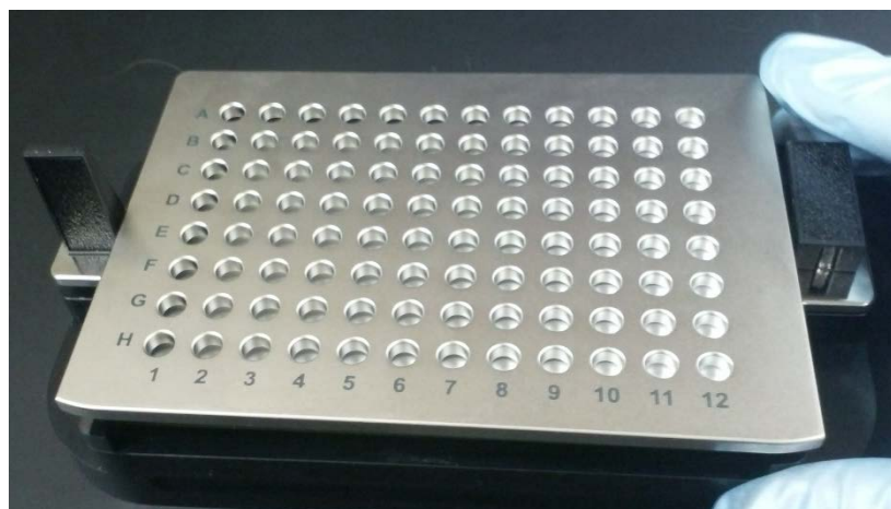
Figure 4: Placement of sealed PCR plate into droplet reader plate holder.
