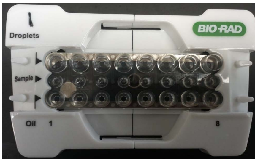
Figure 1: Disposable cartridge properly snapped into droplet generation cassette.
