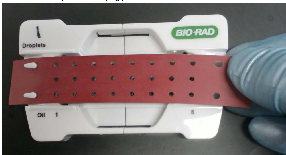
Figure 2: Placement of gasket onto droplet generation cassette.
