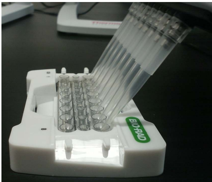
Figure 3: Removal of newly formed droplets with proper pipet tip angle.
