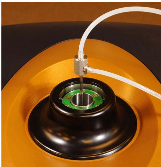
**Figure 18** Tubing connected to cleaning tool.
