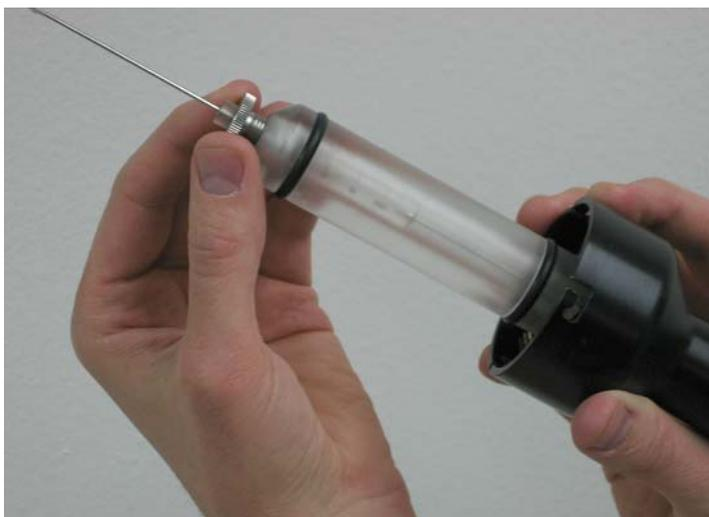
**Figure 15** Tightening the syringe into place.
