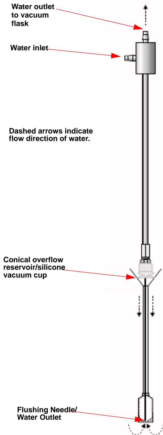
**Figure 19** Side view of cleaning tool in sample cell.
