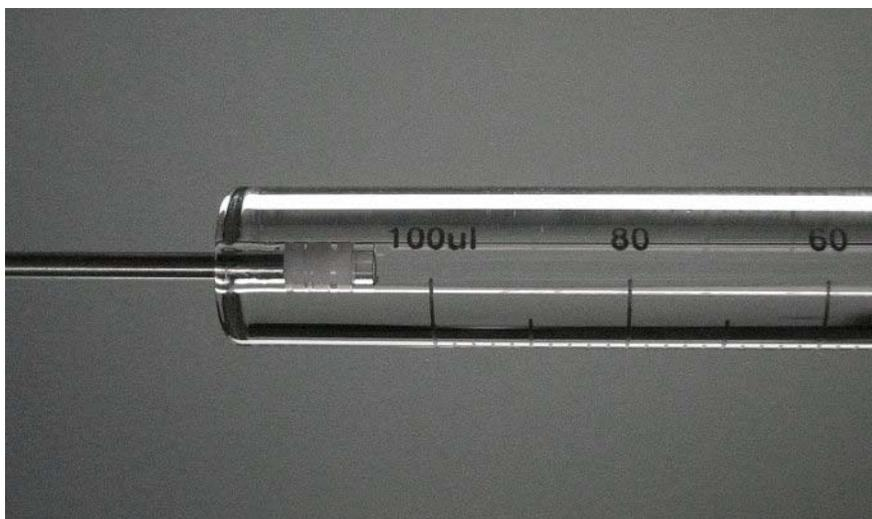
**Figure 13** Syringe with air gap.
