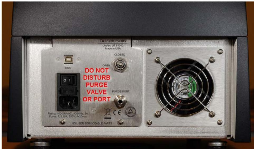
**Figure 21** Location of purge valve and port on rear of instrument.
