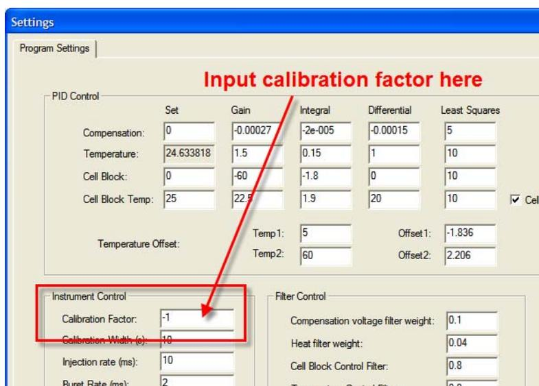
**Figure 10** Calibration factor location.
