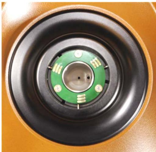
**Figure 12** Sample (center) and reference (right) cell access tubes.
