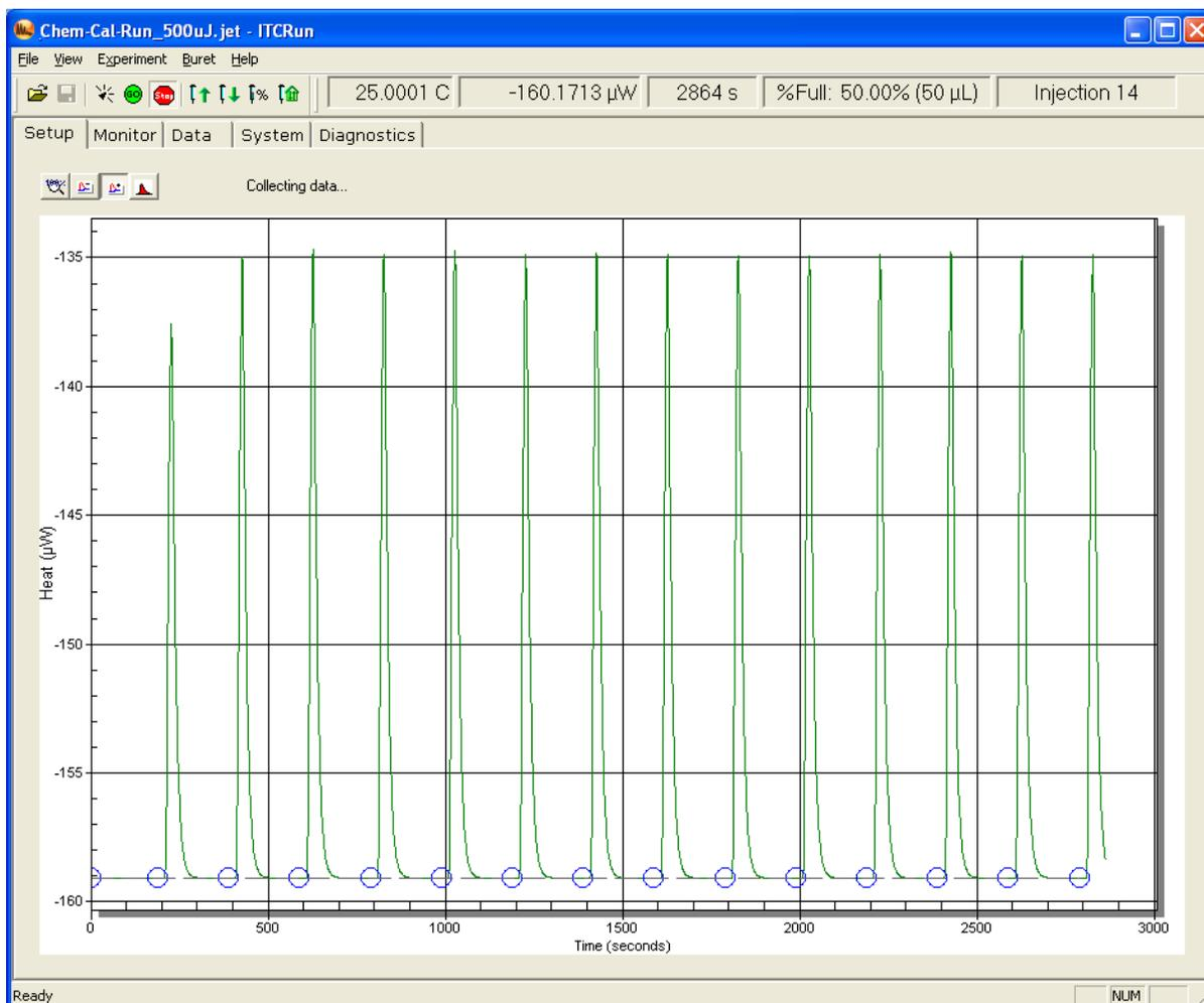
**Figure 9** Example of successful calibration.
