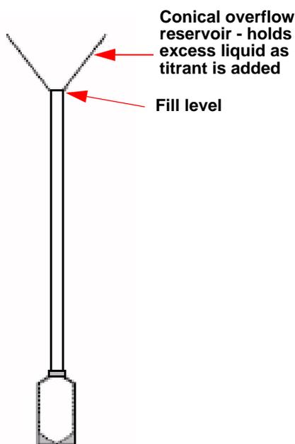
**Figure 11** Side view of sample cell and access tube.
