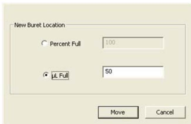
In order to ensure that the reported position of the buret drive matches the actual position, a new **Home Reset** function has been added. This moves the buret drive all the way to the bottom of the stroke in order to find a home reference, then moves the drive upwards by exactly the length of the syringe stroke. Follow the instructions on the screen, paying particular attention to removing the syringe from the buret handle before proceeding.
