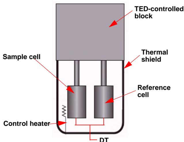
**Figure 4** Nano ITC measuring unit.
